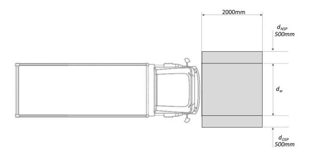
The MOIS shall provide an information signal for VRUs that are stationary or moving forward at speeds of between 3 km/h and 5 km/h when travelling from the nearside or offside of the vehicle in a direction perpendicular to the vehicle median longitudinal plane.
